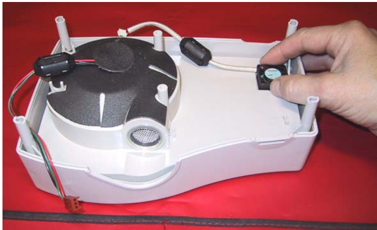
Figure 5-11. Removing the fan from the chassis
