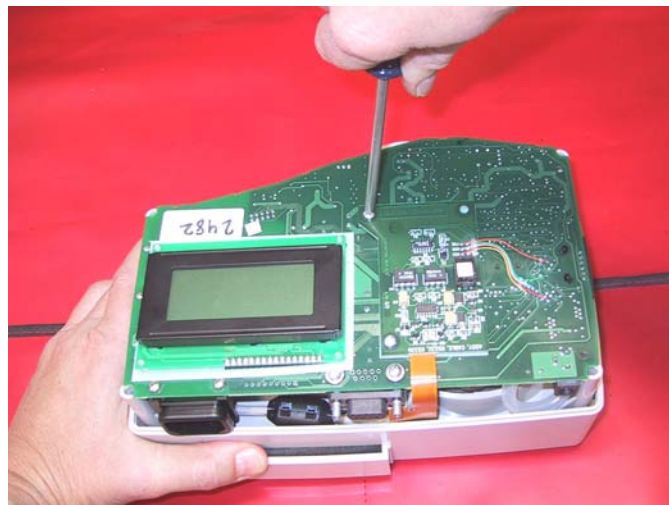
Figure 5-7. Removing the Main PCBA screws
