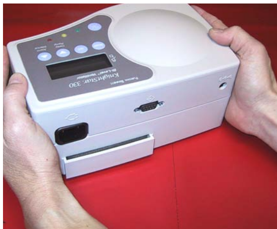
Figure 5-12. Aligning the rear connectors
