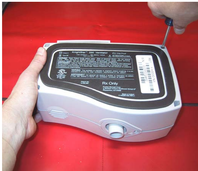
Figure 5-1. Removing the enclosure base screws
