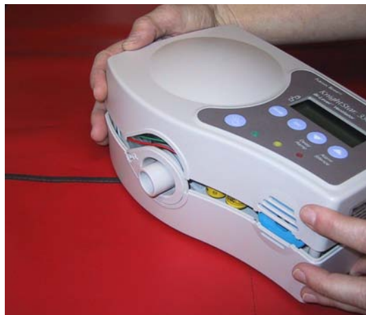
Figure 5-13. Installing the enclosure cover
