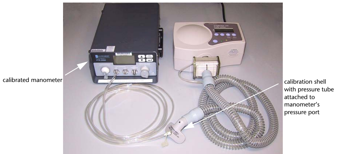
Figure 3-2. KnightStar 330 test set-up
