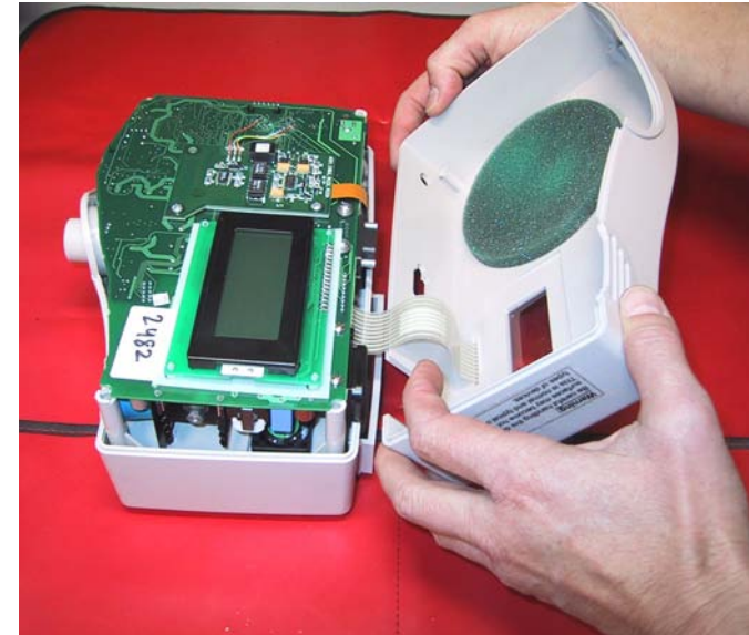
Figure 5-3. Removing the enclosure cover
